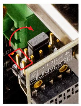
Once the jumper is placed in this position, the gateway **will be factory defaulted immediately.** There is no need to wait 5 seconds. Place the black jumper back in the "**NET**" position (or whatever position it was originally in, if hard-patching Universes), and put the device back in the enclosure.
