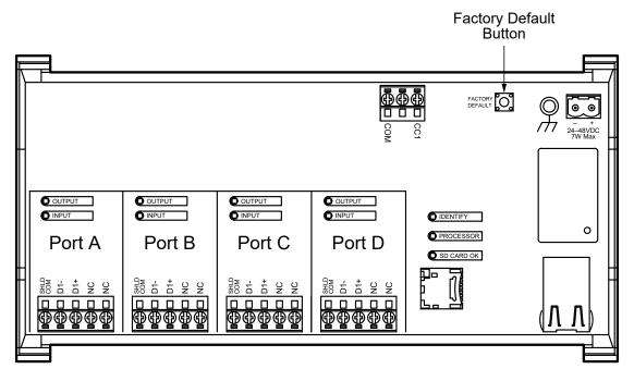
To factory default the gateway, press and hold the button for 5 seconds. This will perform a full factory default.
