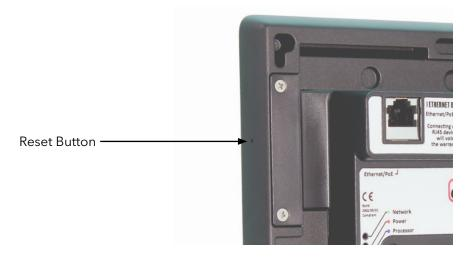
Like the Cognito<sup>2</sup>, insert a USB drive loaded with Choreo firmware into the USB port on the rear of the device. Using a plastic-coated paperclip or similar **non-metallic** small tool, insert it through the hole in the bezel. Press and hold down the button while powering up the Choreo. Keep the reset button pushed until the Choreo shows you the "**System Recsue**" screen.
