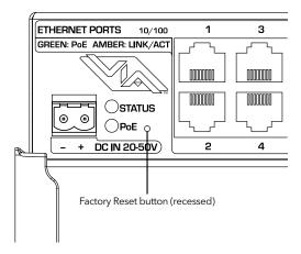
Using a plastic-coated paperclip or similar **non-metallic** small tool, insert it through the hole in the panel. Press and hold down the button for a **full 5 seconds**. **This will perform a full factory default**.
