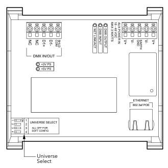
To reset the gateway, set the switches for Universes 1, 3 and 4 to the "ON" position (to the right).
