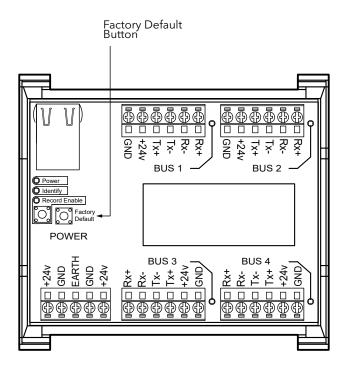
To factory default the device, press and hold this button for a 5 full seconds. This will perform a full factory default.
