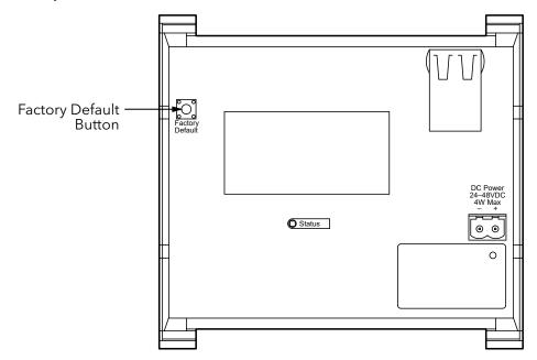
To factory default the device, press and hold this button for a 5 full seconds. This will perform a full factory default.
